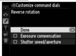
**Change main/sub:** If **Off** is selected, the main command dial controls shutter speed and the sub-command dial controls aperture. If **On** is selected, the main command dial will control aperture and the sub-command dial shutter speed.
